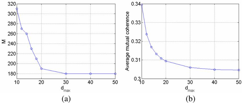
**Figure 12.**  $M$  and TMAC under different value of  $d_{\max}$ . (a) Required  $M$  to achieve acceptable SNR. (b) TMAC when  $M = 210$ ,  $d_{\min} = 10$  m. Note: (a) is obtained by increasing  $M$  so that the lowest SNR is larger than the acceptable SNR 40 dB in 50 repeated simulations.
