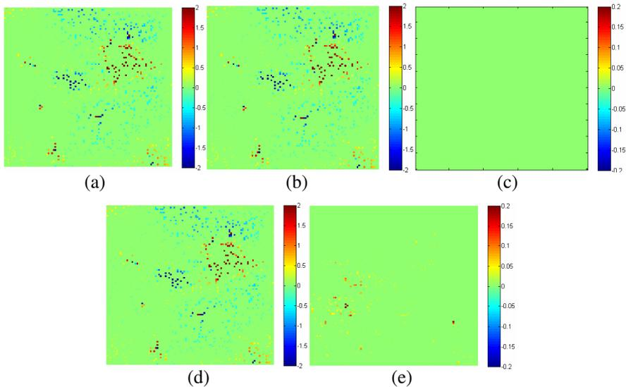
**Figure 10.** The recovery quality when SNR is 40 dB. (a) Original data. (b) Recovered data with SNR 40 dB. (c) Difference between (a) and (b). (d) Recovered data with SNR 30 dB. (e) Difference between (a) and (d).
