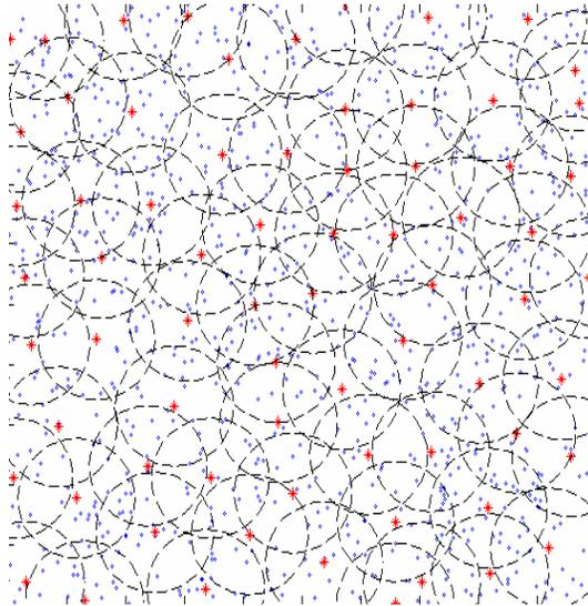
**Figure 6.** Low-coherent Local CIR (LCL-CIR) model. Each circle represents one cluster where “.” denotes the sensor node and “\*” denotes the projection node which is responsible to transmit the measurements of its cluster to fusion center. Note: The locations of nodes are generated as random values drawn from the standard uniform distribution on the open interval (0, 100).
