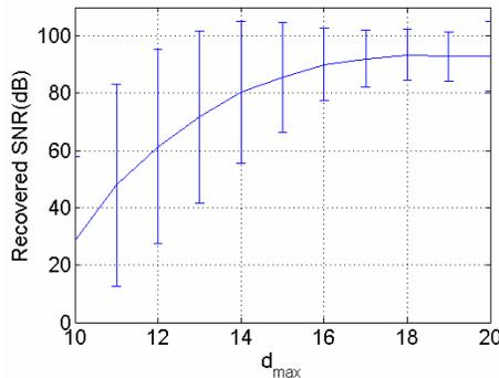
**Figure 13.** Recovered SNR with different value of  $d_{\max}$  when  $M = 210$ ,  $d_{\min} = 10$  m. Note: The error bar shows the variation of SNR with the random locations of  $M$  projection nodes.
