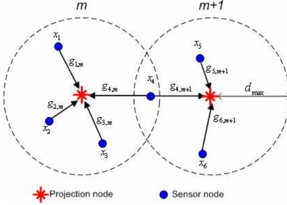
**Figure 7.** Local superposition in clusters. The radius of  $\Omega(m)$  is  $d_{\max}$ . Sensor nodes  $\forall n \in \Omega(m)$  transmit their samples to  $m$ th projection node. Then, Sensor nodes  $\forall n \in \Omega(m+1)$  transmit their samples to  $(m+1)$ th projection node.
