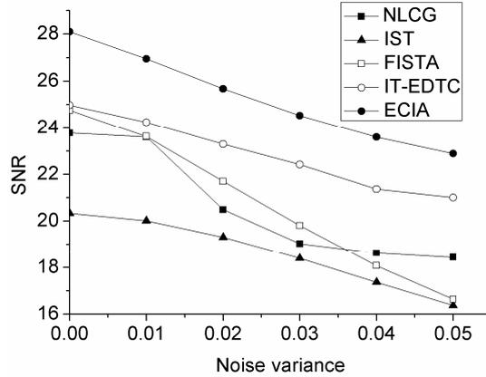
Fig. 7. Curves of SNR versus noise variance of different algorithms.
