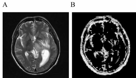
Fig. 3. (A) Original image. (B) The guiding maps for the 3rd scale of à trous WT. The decomposition level is 4.
