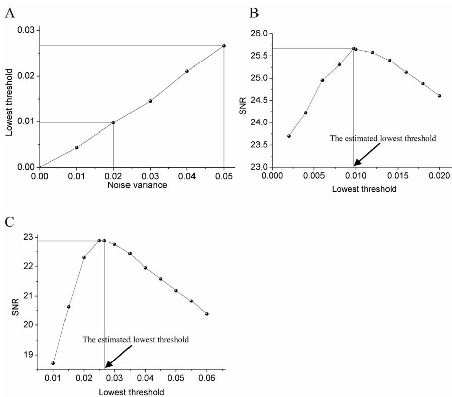
Fig. 8. (A) The curve of estimated lowest threshold versus noise variance. (B) The curve of SNR versus lowest threshold, Gaussian noise with variance 0.02 is added. (C) The curve of SNR versus lowest threshold, Gaussian noise with variance 0.05 is added.
