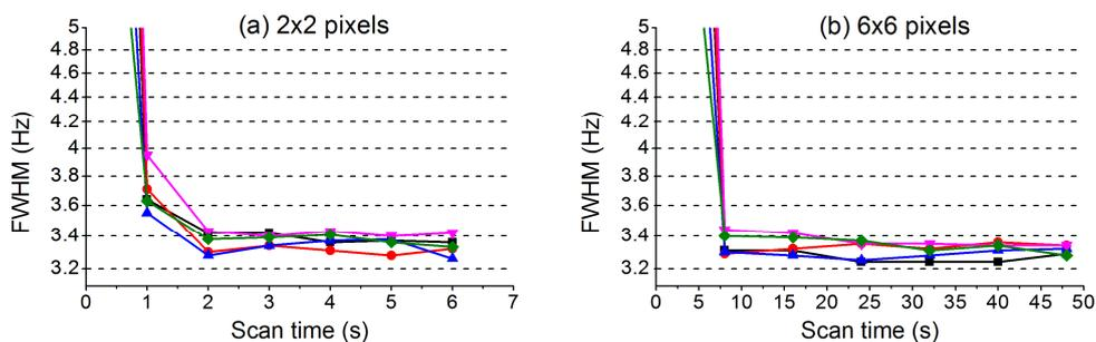
Fig. 7. The  $^1\text{H}$  gradient shimming with  $2\times 2$  pixels and  $6\times 6$  pixels on the doped 4 Hz  $\text{H}_2\text{O}/\text{D}_2\text{O}$  sample. Lines dotted with (■), (●), (▲), (▼), and (◆) are initialized from the same shim values as those used in the  $^2\text{H}$  shimming (Fig. 6).
