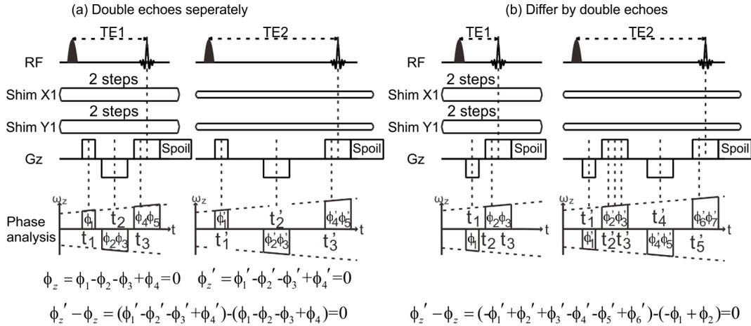
Fig. 3. Two improved  $^1\text{H}$  sequences to compensate thermal convection. (a) Both two imaging scans utilize the double gradient echoes; (b) two imaging scans differ by double gradient echoes.
