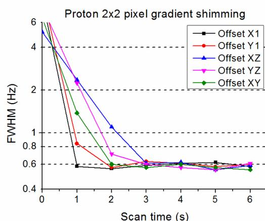
Fig. 5. Results of 2×2 pixel  $^1\text{H}$  gradient shimming that is initialized by offsetting one of off-axis shim coils. The test sample is the mixture of DMSO (500  $\mu\text{L}$ ) and DMSO- $\text{d}_6$  (100  $\mu\text{L}$ ) containing 0.05% TMS.
