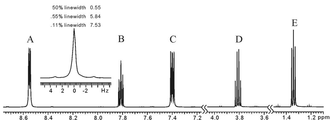
Fig. 8. A <sup>1</sup>H NMR spectrum obtained from selective 2×2 pixel <sup>1</sup>H gradient shimming. The test sample is the mixture of pyridine (150 μL) and alcohol (50 μL) in D<sub>2</sub>O (200 μL) containing 0.05% TMS. The FWHM of the TMS peak after shimming is 0.55 Hz in the inset graph. The center frequency of the selective RF pulse can be moved to any peak among A ~ E.
