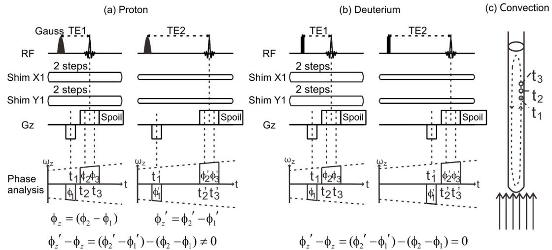
Fig. 2. (a)  $^1\text{H}$  pulse sequence with a Gaussian RF pulse. (b)  $^2\text{H}$  pulse sequence with a hard RF pulse. The separations of dephased and readout gradients are different between  $^1\text{H}$  and  $^2\text{H}$  sequences. (c) Thermal convection in the sample caused by the VT airflow. When a magnetization
