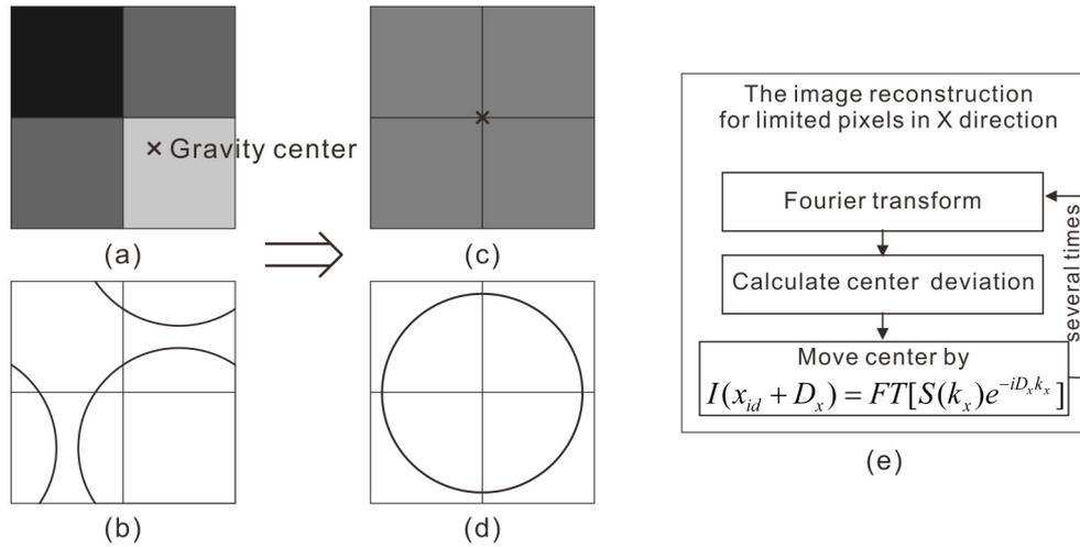
Fig. 1. (a) The image with different intensities in different regions after Fourier transform, (b) an illustration of the sample deviating from the FOV center, (c) the image with uniform intensity after correction, (d) an illustration of the sample located at the FOV center, and (e) the image reconstruction process.
